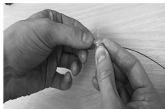
2 Gently push the cleaning wire through the tubing from top to bottom. Pull the cleaning wire all the way through.
