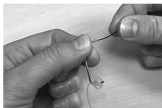
3 Remove any debris from the end of the tubing and wipe the dome to remove any excess wax.
